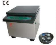
It is controlled by micro-computer and has digital display and electric lock, with the advantages of elegant design, stable performance, high capacity, low noise and low cavity warming. It is suitable for the separation of suspended substances from liquid (e.g. blood plasma) in research institutes of biology, chemistry, public health, medicine, food and environment protection.
