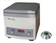
It is made of high strength plastic, easy to operate and suitable for qualitative analysis of blood serum, blood plasma and radio-immunity in hospitals and biochemical laboratories.
